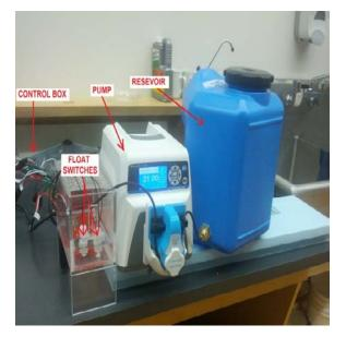
Figure 1 - Humidification System Components of the occupant simulator system [34]
