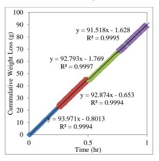
Figure 6 - Calibration of box 1111: Run #3
