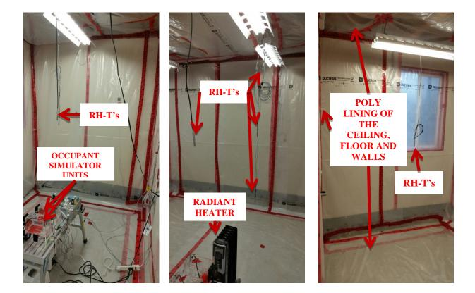
Figure 9 - Experimental setup of the WBPRL for field verification of the moisture production rates of the occupancy simulators
